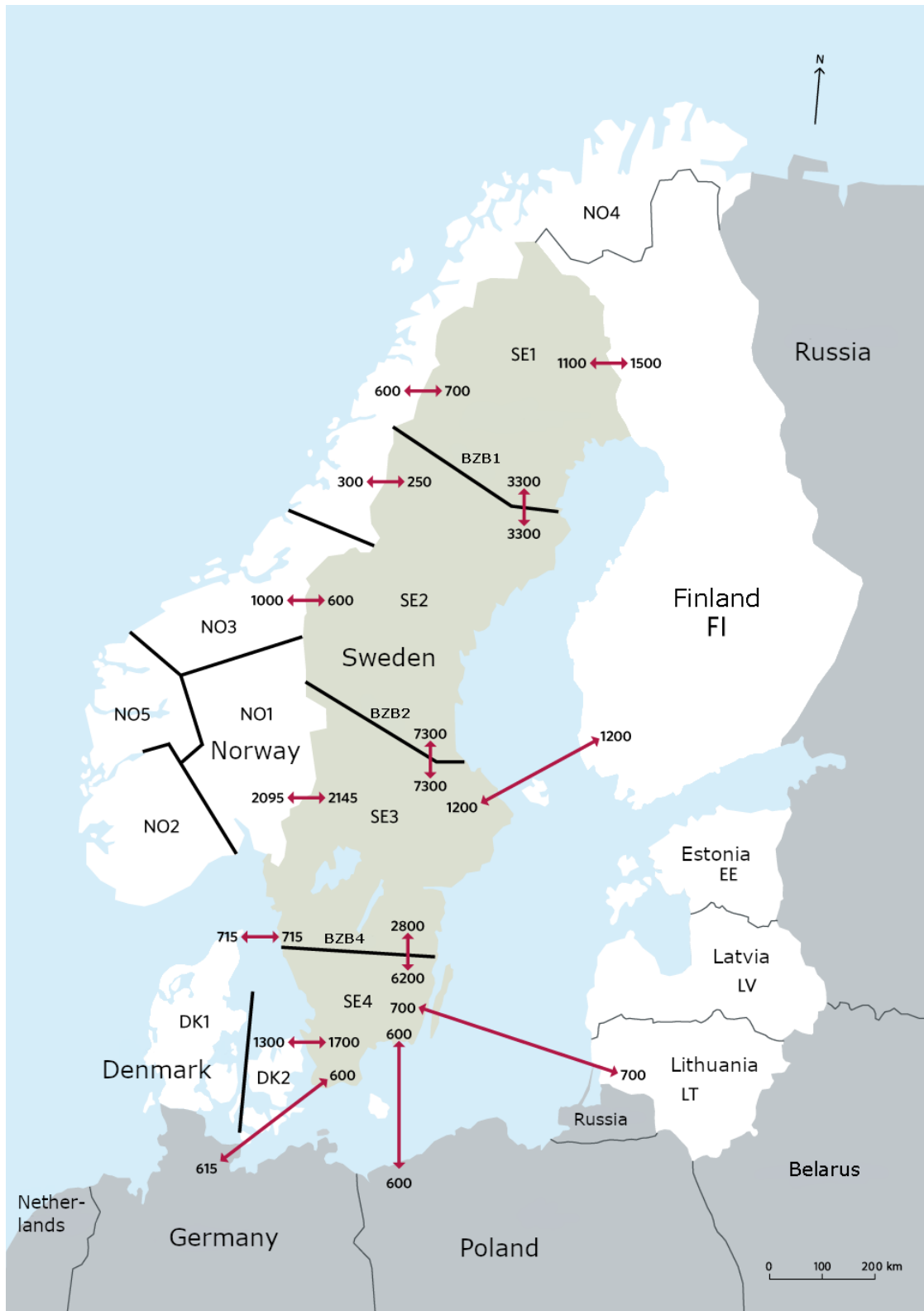
Figure 2.4: BZs in the Nordic synchronous area and current transfer capacities between them [7].
